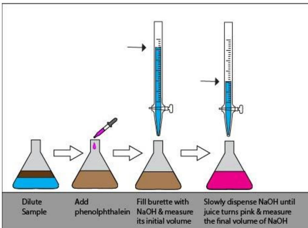
**Figure 2: Steps of acid titration**
